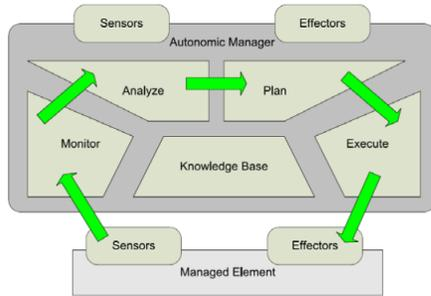
Figure 2: The MAPE-K loop (Image from [29]).
