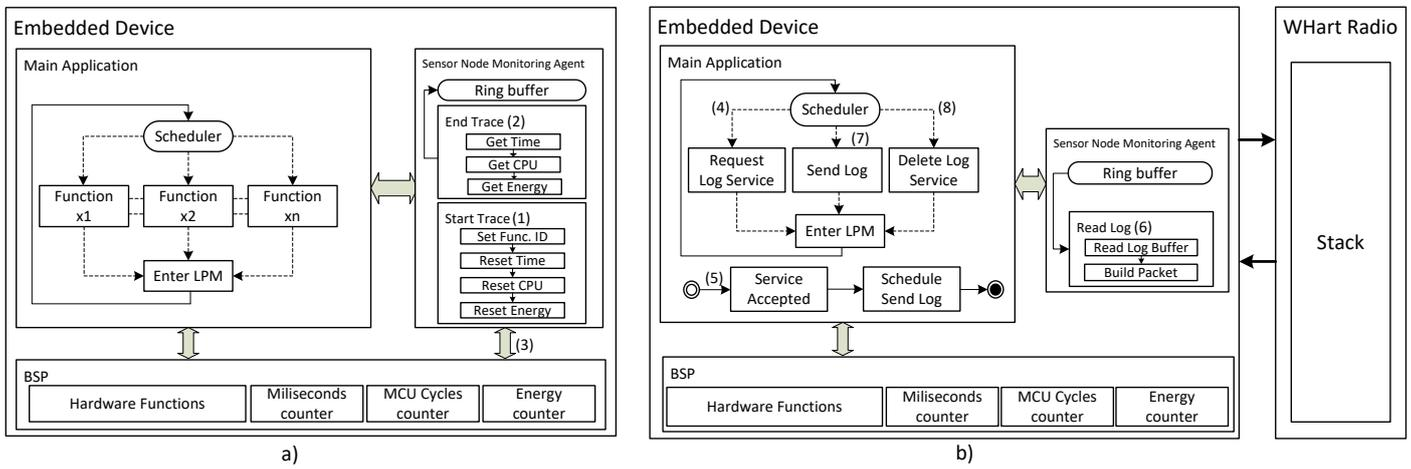
Figure 2- On the left, (a) the application architecture and the sensor node monitoring agent acquiring the state information. On the right, (b) the request of the WirelessHART publish service
