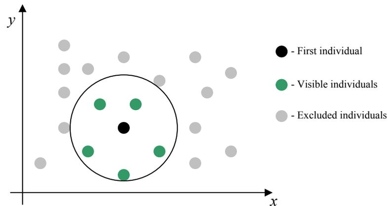
Figure 2 - Selection mechanism: visibility radius
