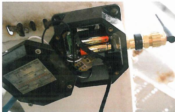
Fig. 4. Sensor node in an ATEX junction box.
